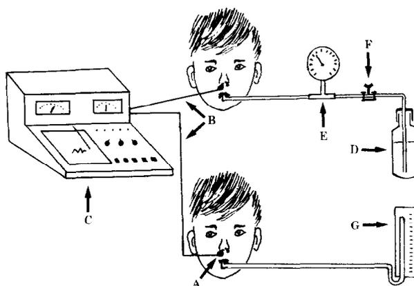
Fig. 1. Manometric measurements of pressure gradients developing within the nasopharynx and oral cavity: during forced sucking (top), and during forced blowing (bottom): A: the probe is applied to the funnel connector of the catheter. B: the electrical cord to the pressure transducer (C). D: the water bottle from which the patient is sucking water through an elastic tube. E: negative pressure manometer connected by a T system. F: laboratory compression screw. G: blood pressure sphygmomanometer.
